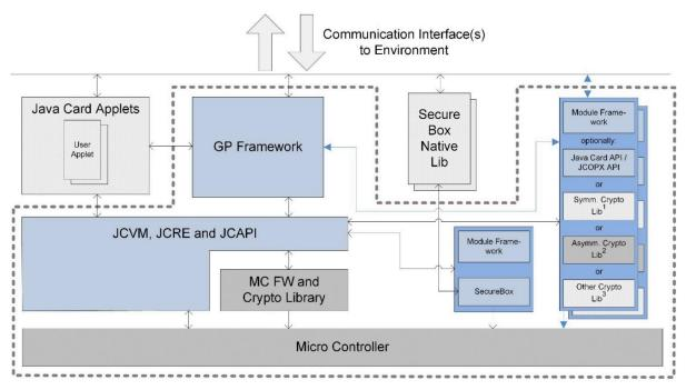
In the above figure, the blue parts are in scope of the TOE, with the items in darker grey being provided by the composite (certified hardware and crypto library). The items in light-grey are out of scope.
